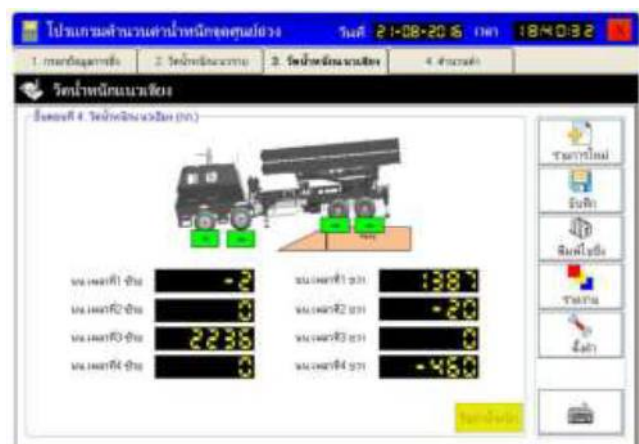
Fig. 2 the final result of the CG measuring software
